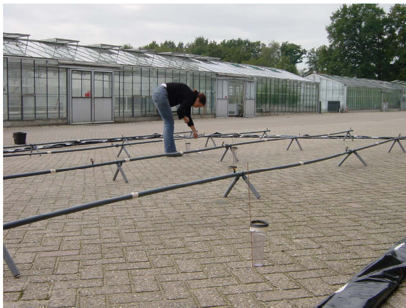
Plate 4. Pluviometers placed diagonally across the field.
