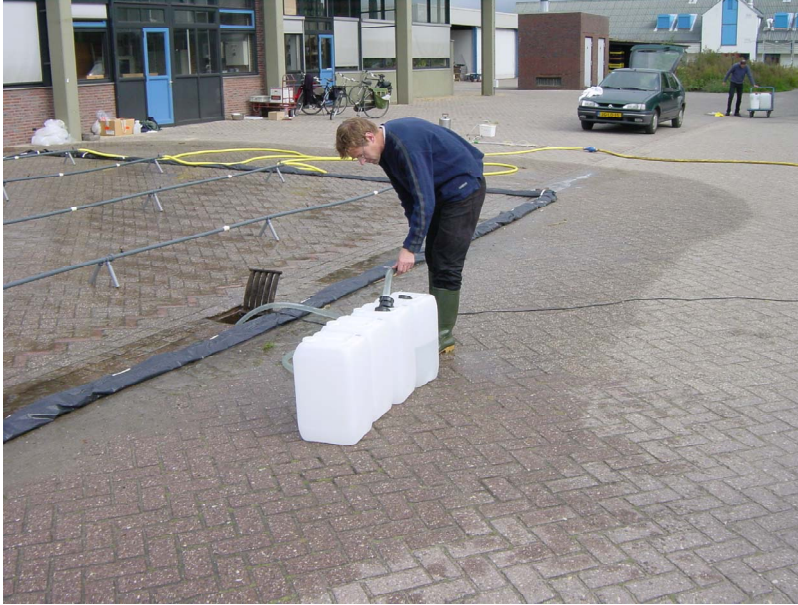
Plate 3. Pumping runoff water into PVC containers.
